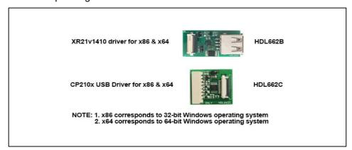
Figure 1.3 Serial port driver
