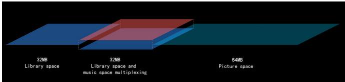
Figure 2.2 128 MB memory space diagram
