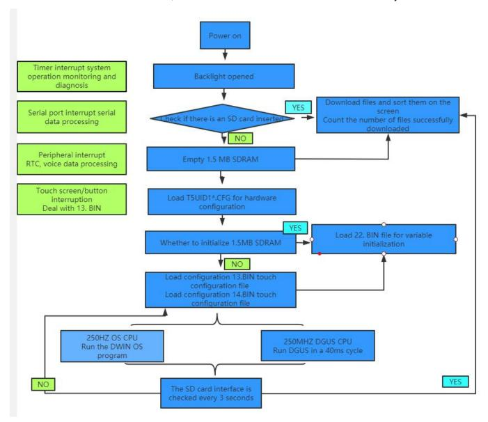
Figure 2.1 T5UID1 DGUS operation flow chart
