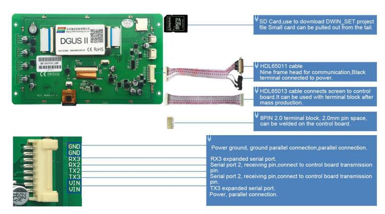
Figure 1.2 8 pin 2.0 interface definition and wiring description
