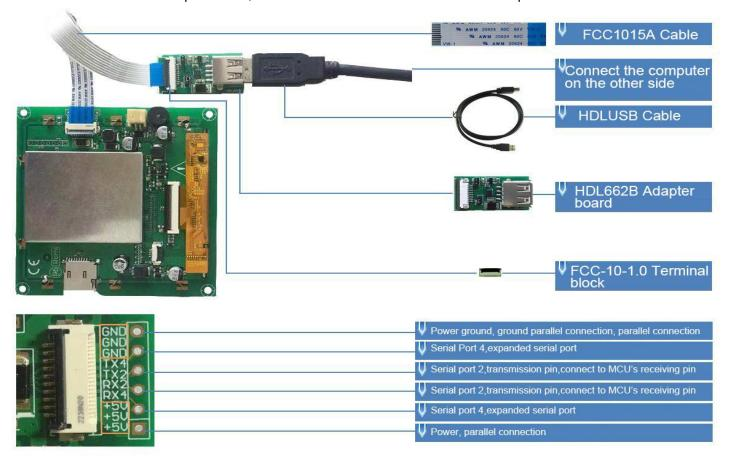
Figure 1.1 10 PIN interface definition and wiring description
